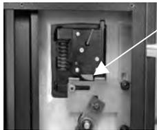
3. Make sure there is a minimum clearance of 0.150 inch (3.8 mm) between the end of the lock case and the blocking bar of the safe's boltwork.
