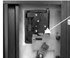
5. The lock cannot function properly if it binds against the safe's boltwork. This photo shows boltwork in the fully locked position, placing pressure on the side of the lock bolt. It could prevent the lock from opening.
