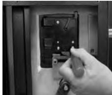
2. After making sure the cable is protected within the lock's recessed channel and not crimped or stressed at any point, attach the lock body to the mounting surface using the screws provided. Tighten the mounting screws to 30 to 40 inch-pounds (33.9 to 45.2 dNm).
