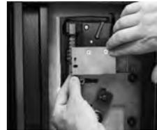
4. If the safe incorporates a relock device plate, it will likely attach to the lock body as shown. If it attaches using the lock's cover screw, make sure the screws engage the lock by at least four threads. Substitute longer 8-32 machine screws if necessary. It may be necessary to trim longer screws to a proper working length. Relock device attaching screws must NOT be longer than the depth of the tapped hole provided in the lock case.
