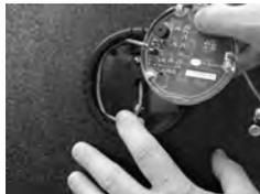
12. The lock cable should be routed inside the keypad assembly as shown in the photo. Make sure the cable is not crimped or pinched.
