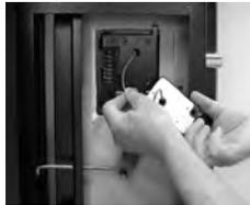
1. The mounting surface should be smooth and flat, with either 1/4-20 or M6 mounting screw holes. The wire channel (spindle hole) through the safe door must be at least .312 inch (7.9 mm) in diameter. Insert the lock cable through the spindle hole and gently pull it from the front of the safe as you place the lock body against the mounting surface.
