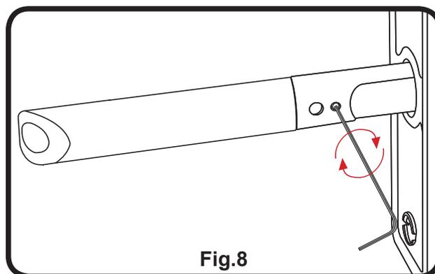
6. Adjust the latchbolt to the desired length by rotating it anti-clockwise to increase the length between 115mm-130mm. When at the desired length, using the 4mm (3/16") hex key, replace the hex head bolt located in the end of the latchbolt as per **Fig.9**.
