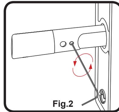
2. Using a 4mm (3/16") hex key, remove the hex head bolt located in the end of the latchbolt as per **Fig.3**. Keep this bolt, as this will be needed when the XL latchbolt is fitted.
