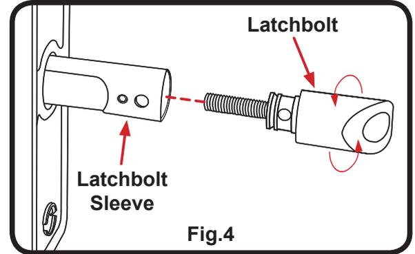
4. Ensure that the 2 x ball bearings are in line with the holes either side of the XL latchbolt as per **Fig.5**. If there is not already - place a small amount of grease around the ball bearings to ensure they do fall out of the holes. With the bearings in position, screw the threaded part of the XL latchbolt (clockwise) into the latchbolt sleeve until both halves join as per **Fig.6**.
