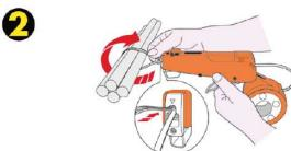
Wrap the strapping around the item(s) to be bundled with the serrated surface up. Insert the end of the strap into the locking clip until an audible "click" is heard.
