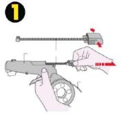
Remove the spring feeding guide by squeezing both sides of the locking end cap.
