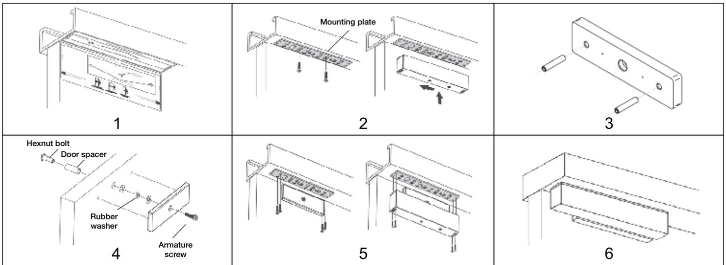
1. Use the supplied template to determine the correct location and size of mounting holes for both the door and frame header. Ensure that the door opens away from the maglock. In the case of a single door, the maglock is positioned as close as possible to the vertical section of the door jamb. Drill door and frame as indicated.
