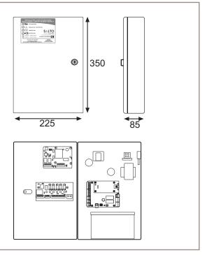
The PB212S is a monitored Linear Power Supply designed to power and protect SALTO Control Units. It permits the connection of the control unit to other equipment used in the security, fire, CCTV and access control industries.
